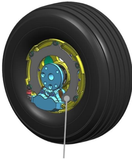
Brake disc type A3 (thickness 3 mm)
