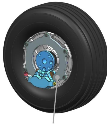
Brake disc type A8 (thickness 8 mm)
