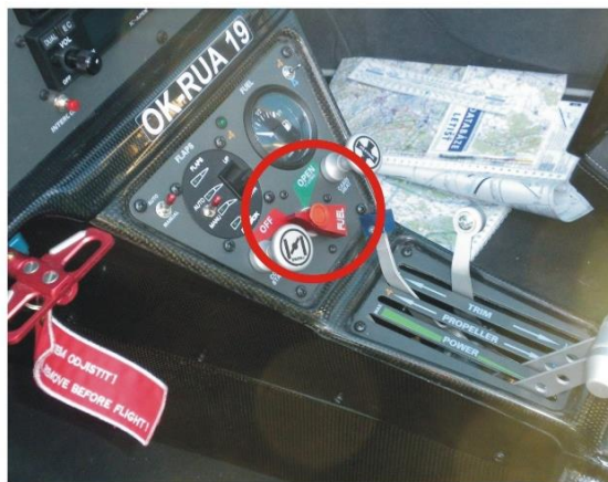
TL - ultralight two - way Fuel shutoff Valve
