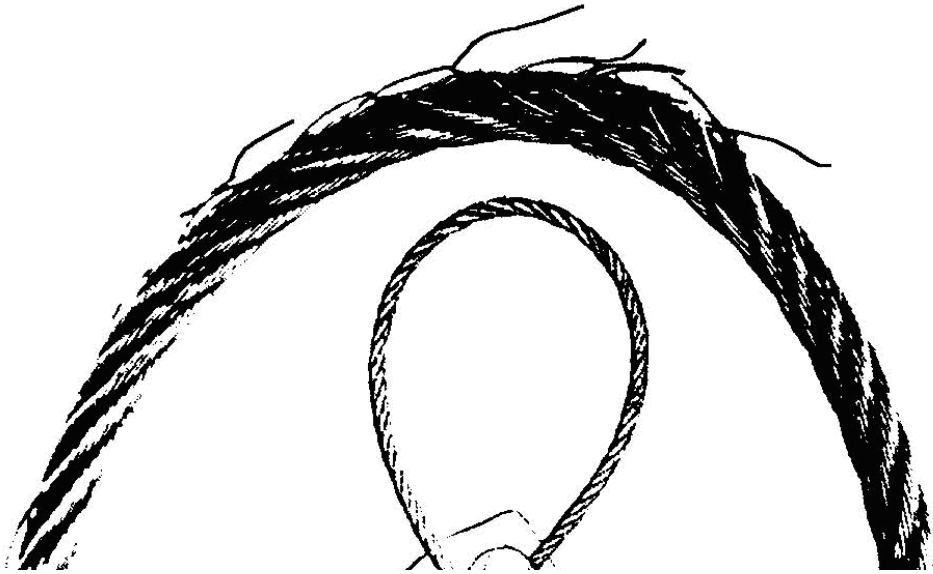
Figure: Wire cable strands exposed by bending the cable.
