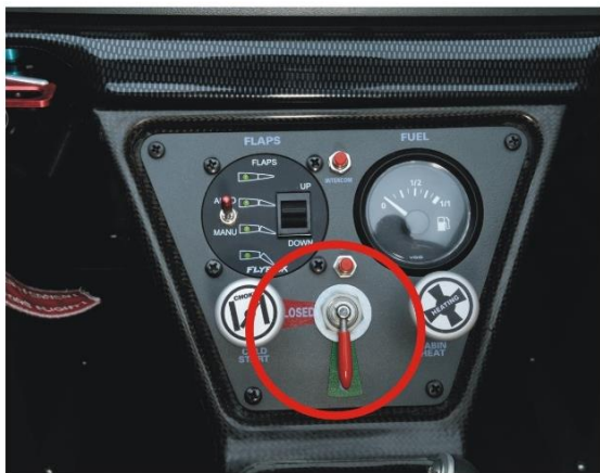
22 MB two - way Fuel shutoff Valve
