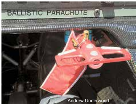
Such safety devices are becoming increasingly common on LSAs and GA aeroplanes alike.
