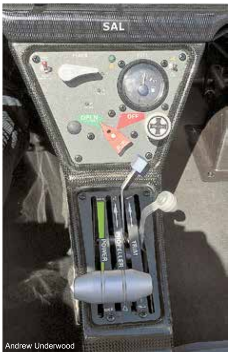
Andrew Underwood The Sting's centre console has all the primary controls grouped neatly, including fuel.
