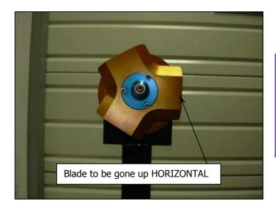
Position the hub of the propeller with variable pitch on a support so as to obtain a horizontal position of the blade to be gone up.
