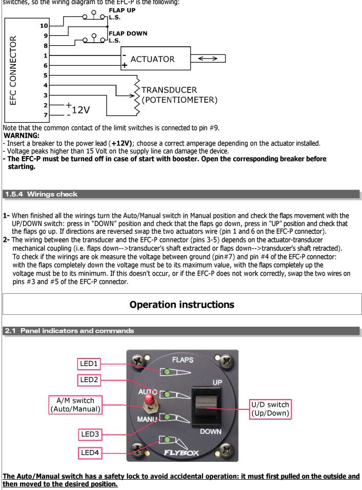
The EFC-P can work in two modes: Automatic or Manual.
