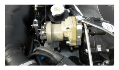
Picture no. 5 PowerMax pitch control hydraulic governor
