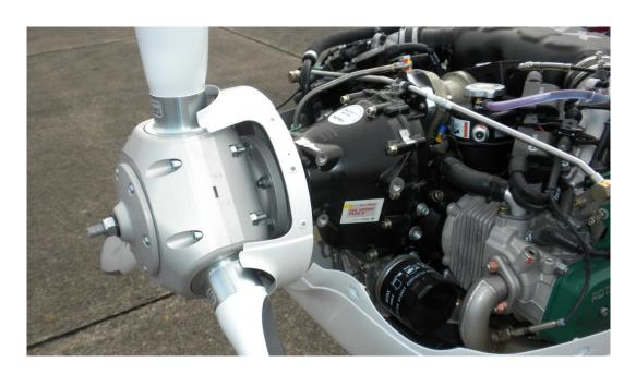
Picture no. 17 Propeller installation onto the propeller boss
