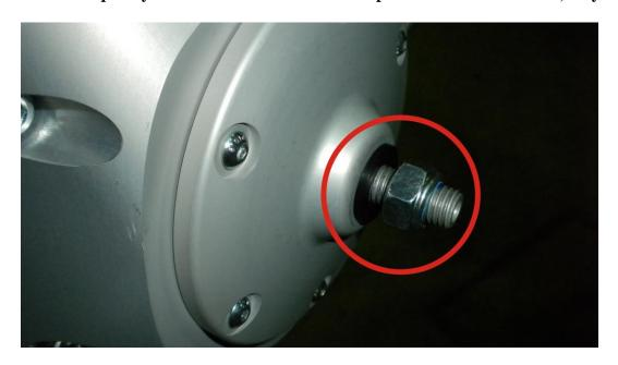
Picture no. 18 Nut M 12 releasing
