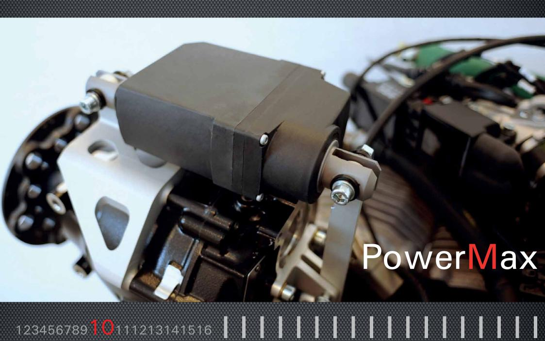
I The highly reliable electric motor is used to adjust the blade pitch. It guarantees trouble-free operation even after hundreds of thousands of operational cycles.
