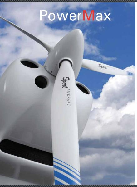
I The all-composite propeller blade is manufactured from carbon fibre, the hub and pitch control mechanism from the highest quality superdural alloys. The strength and resistance of the PowerMax propeller was confirmed during stringent certification tests. Eg. the strength of the blade corresponds to seven times the maximum permissible operational loading (which means the tensile strength of each blade is more than 10,5 tons).
