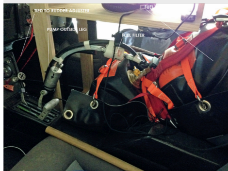
Supplementary fuel system setup.
