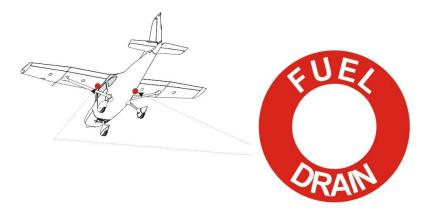
Around venting of fuel tanks on the bottom side of the wings:
