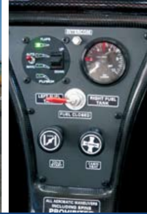
Above, left: Attractive side profile of the Sirius. Above, middle: Foolproof fuel and flap controls on the centre console. Above, right: The Dynon 100 EFIS and Garmin 695 GPS fitted to ZK-SPR.
