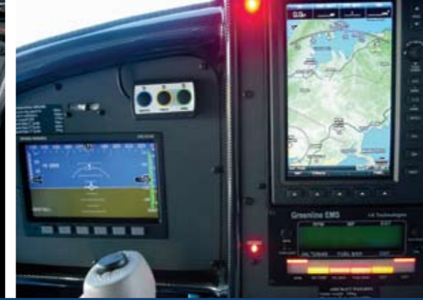
Above, left: Attractive side profile of the Sirius. Above, middle: Foolproof fuel and flap controls on the centre console. Above, right: The Dynon 100 EFIS and Garmin 695 GPS fitted to ZK-SPR.
