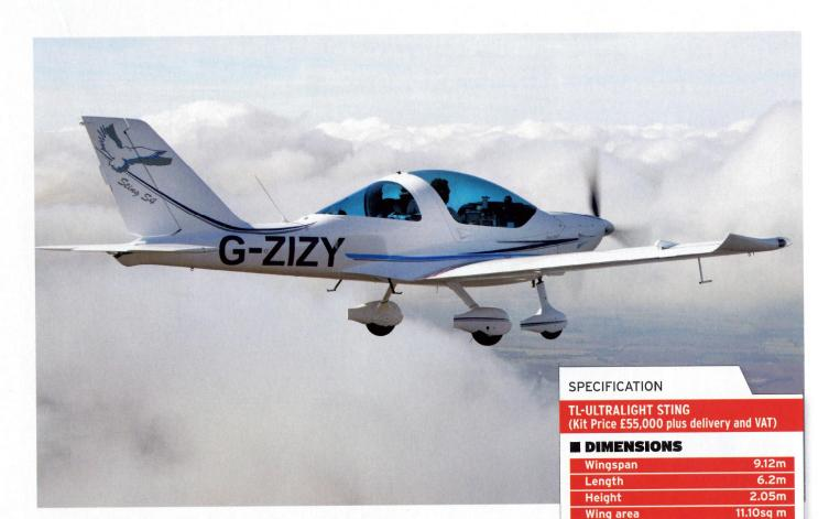
and anyway I doubt that it would normally ever be an issue (my test represents a fairly extreme condition). Slowing down to assess the low-speed end of the flight envelope confirms that the Sting is as slippery as it looks, as it takes a while to reduce speed. Slow flight is very benign and stalls are an absolute doddle, whether
