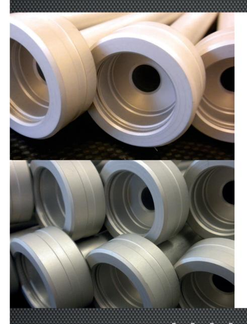
I Modern CNC technologies are used to their maximum in both the design process and during production. These advanced technologies provide high precision and outstanding manufacturing quality. This state of the art high technology and innovative design has enabled the weight to be reduced to an almost unbelievable 8,7 kg – unheard of in this category of in flight adjustable propellers.
