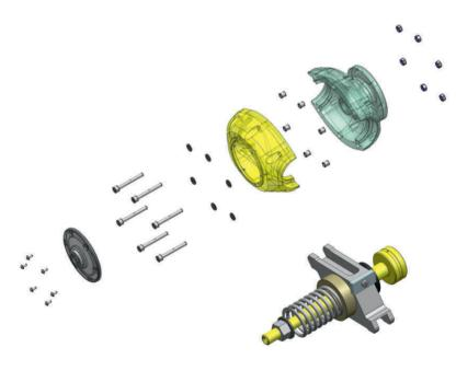
The composite propeller blade is manufactured from carbon fibre, the hub and pitch control mechanism from the highest quality superdural alloys. The strength and resistance of the DuoMax propeller was confirmed during strigentcertification tests. Eg. the strength of the blade corresponds to seven times the maximum permissible operation loading (which means the tensile strength of each blade is more than 12 tons).
