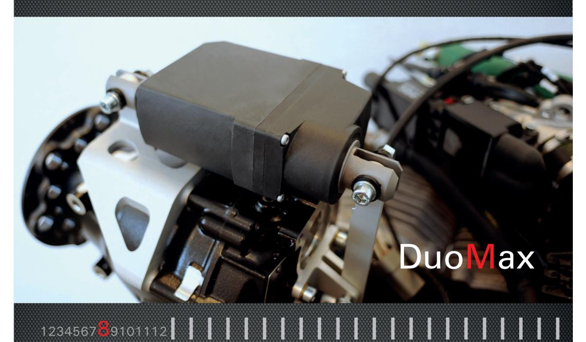
I The highly reliable electric motor is used to adjust the blade pitch. It guarantees trouble-free operation even after hundreds of thousands of operational cycles.
