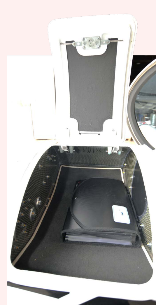
Baggage spaces fore and aft allow you to control the C of G
