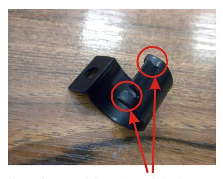
The metal lugs on the support, which is used to grip the flap drive torque tube, may be excessively bent, causing operational damage to the torque tube.
