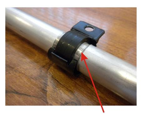
Damage/groove in flap drive torque tube
