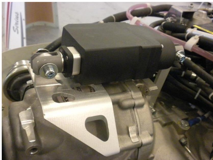
Picture no. 9 Servo motor with holder - assembly
