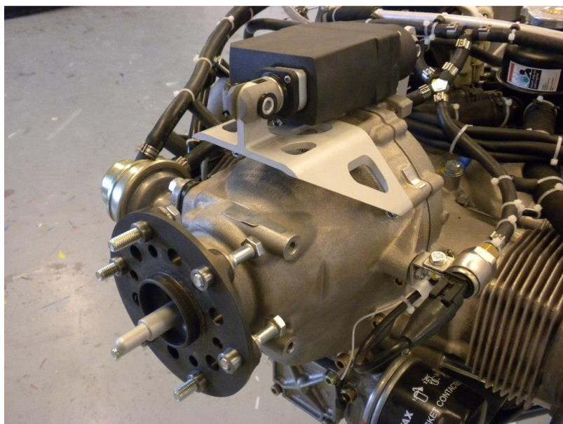
Picture no. 13 Propeller control axis – installation
