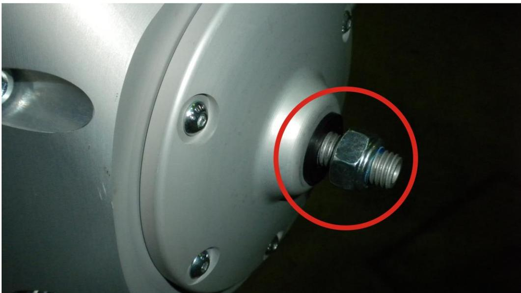
Picture no. 18 Nut M 12 releasing
