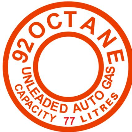
Around wing tank caps: (if installed) (gallons or liters - as required)
